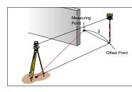
The Series 10 calculates the angles and distance, or the coordinates of the measuring point by inputting the distance and direction between the measuring point and the offset prism.
